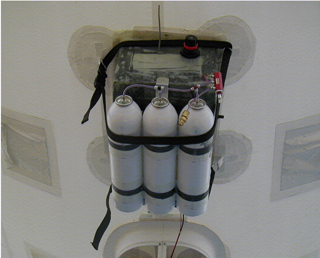
Figure 4. Photograph of Real-time SF 6 Instrument
